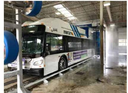
Transit-Master. For buses with front mounted bicycle racks. Dryer system.
